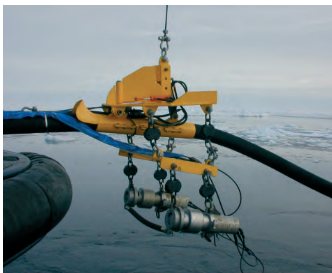
Fig. 5. Airguns with depressor for acquiring seismic data used by the icebreaker "Oden" in the Nansen Basin. Technical solution tailor-made by the University of Bergen.
