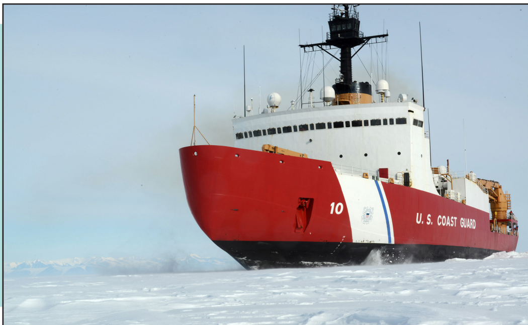
The Coast Guard Cutter Polar Star, with 75,000 horsepower and its 13,500-ton weight, is guided by its crew to break through Antarctic ice en route to the National Science Foundation’s McMurdo Station, Jan. 15, 2017. The ship, which was designed more than 40 years ago, remains the world’s most powerful non-nuclear icebreaker. (Source: US Coast Guard via Flickr, Public Domain)
